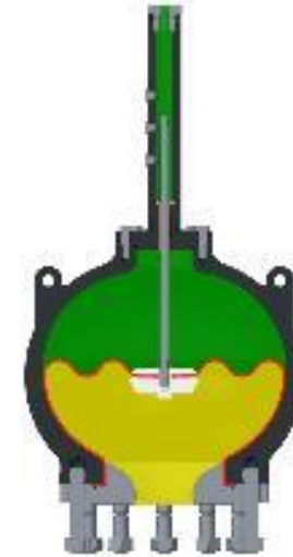
Bladder type discharge dampener for pressures up to 35.000 kPa, to protect pump and pipeline
