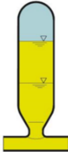
Airvessel type suction dampener for pressures up to 1.000 kPa, to reduce NPSHr
