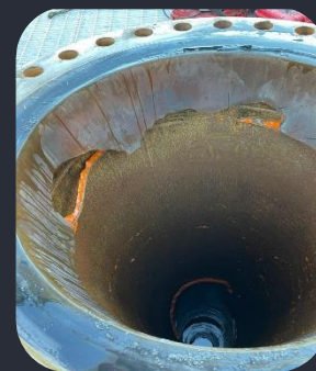
Special Part Failures: Damage to internal linings.
