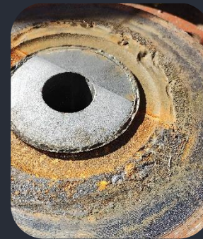
Discharge Ring Failure: Wear, cracking, or breakage of ceramic components.
